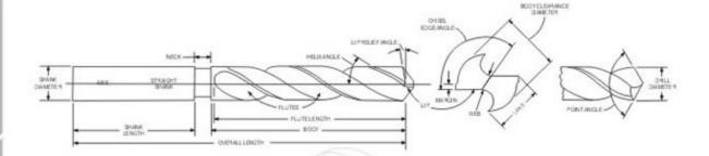
Axis The imaginary straight line which forms the lengthwise center of a drill.
